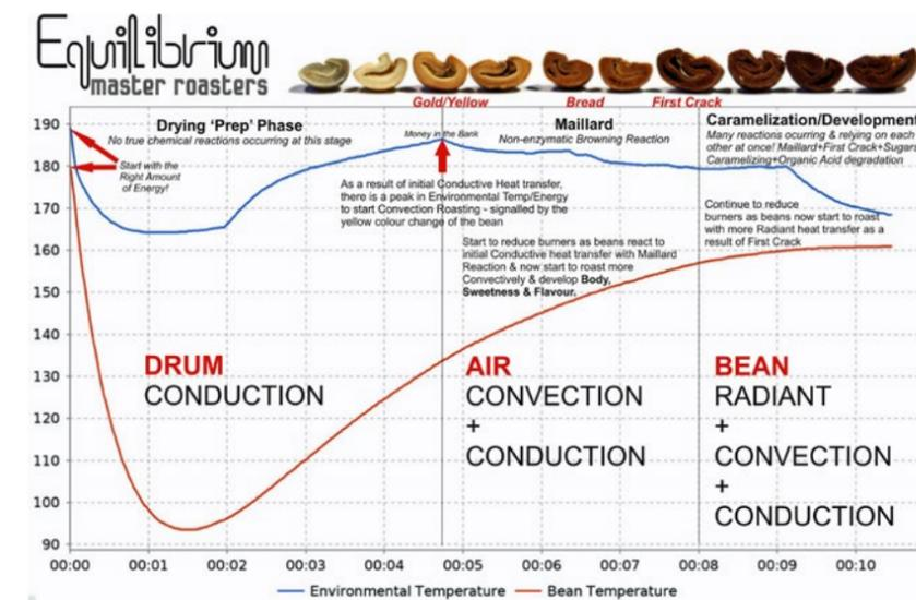
manipulate the rate of convection (HT) in order to control the total energy (& overall profile of the roast) lessening the impact of the Radiant (bean-to-bean) energy of the exothermic beans.
